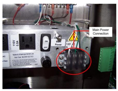
Figure 6. Neutral - Ground – Line Connections
