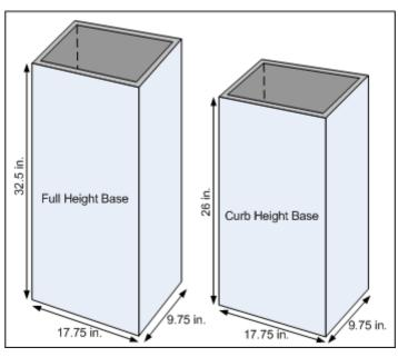
Figure 3. Straight Bases Dimensions
