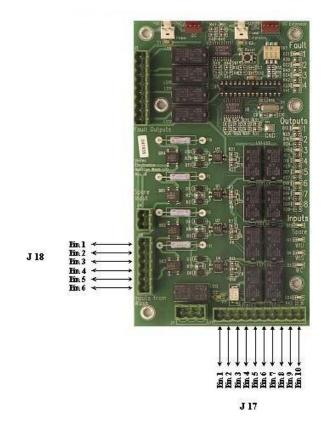
Figure 7. Wash I/O Board Connector Pinouts
