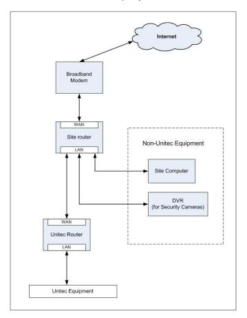
When a router (or modem with built-in router) is used between the Unitec router and broadband connection, it must be configured to allow external connections to and from the C-Start. The router should be configured to:
